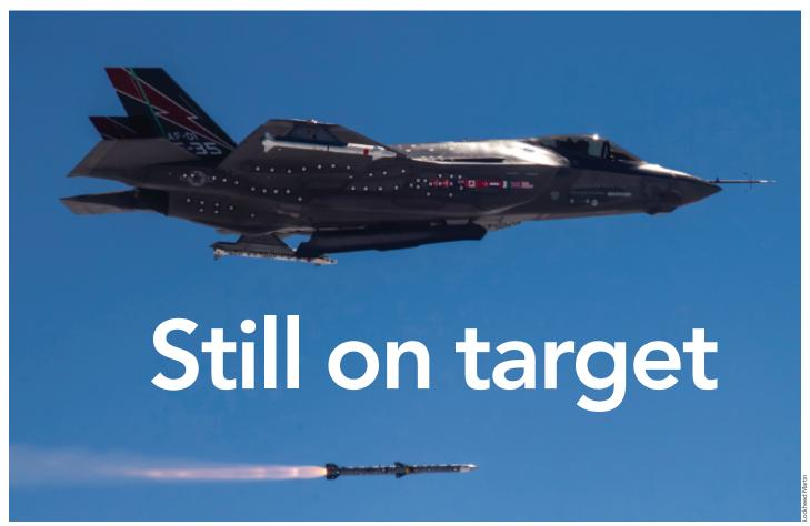
Developed continuously since the mid-1970s, Raytheon's AIM-120 remains a crucial combat capability, including for the stealthy F-35
